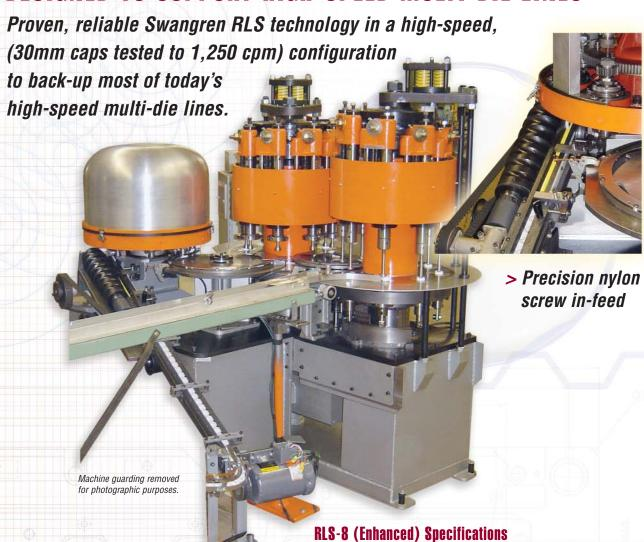
> Main gearing runs in enclosed oil bath
